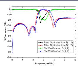
The optimized layout obtained from EMOptimizer\* is exported to UltraEM\* for rigorous EM simulation and verification. The EM simulation validates that the final layout design meets the design specifications.
