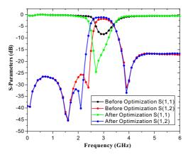
The figure depicts the simulation results of the designed filter before and after EMOptimizer\* performs optimization. After optimization, the passband increases from 2.8GHz-3.2GHz to 2.6GHz-3.2GHz, the insertion loss decreases from 1.8dB to 1.1dB, and the return loss increases from 8.3dB to 17.3dB.
